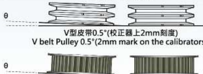
同步皮带 0.25° (校正器上 1mm 刻度) Timing belt Pulley 0.25° (1mm mark on the calibrators.)
